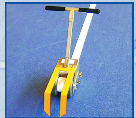
Marking head with guiding for straight lines.
